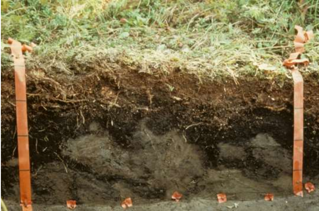
Profile of a Histel (specifically a Fibristel) in Alaska. The organic soil material (brown and black) ranges from about 20 to 40 cm in thickness and is intermingled with the underlying mineral soil material due to cryoturbation. Permafrost is at a depth of about 40 cm. Scale is in decimeters.
