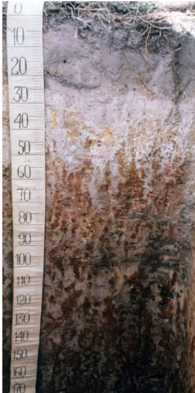
Profile of an Aquult (specifically a Plinthaquult) in Venezuela. Some of the red bodies in the subsoil are plinthite. Scale is in centimeters.
