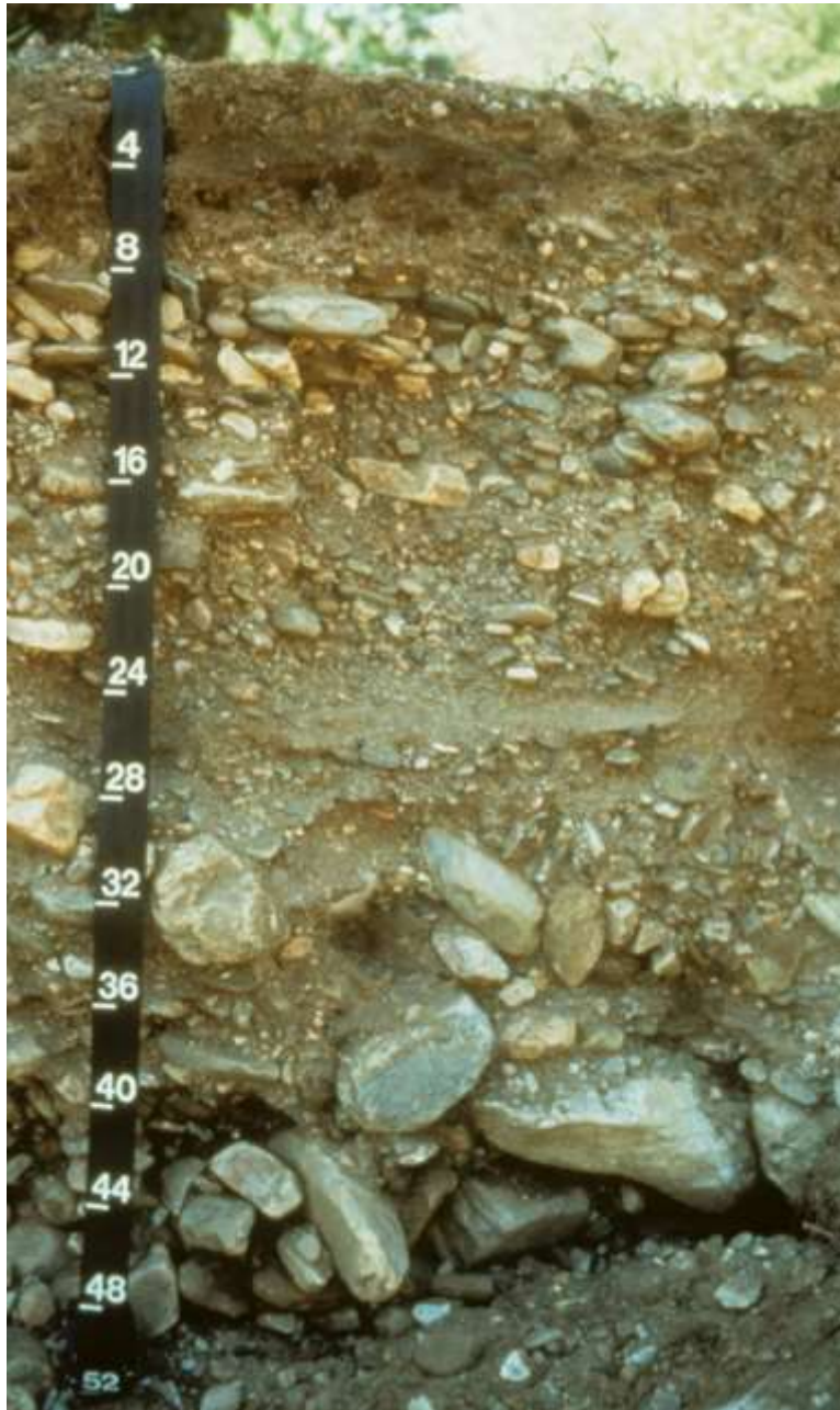
Profile of an Orthent (specifically a Udorthent). This soil formed in gravelly, cobbly, and stony colluvium. Other than the ochric epipedon, this soil has no other diagnostic horizons. Scale is in inches.
