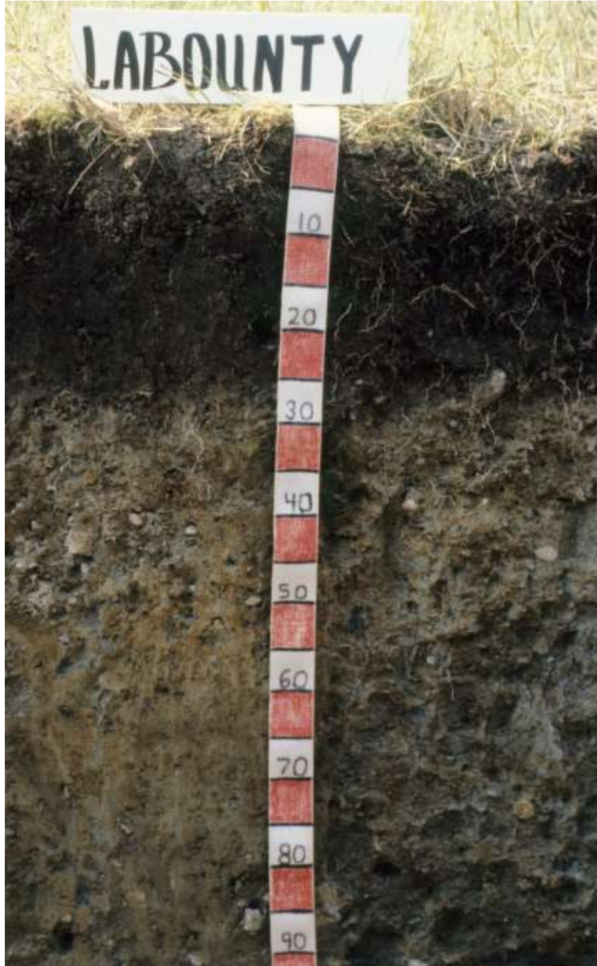
Profile of an Aqualf (specifically an Endoaqualf) in Wyoming. The dark surface layer is an umbric epipedon. The subsoil has the characteristic gray and red mottled color pattern indicating the presence of aquic conditions. Scale is in cm.
