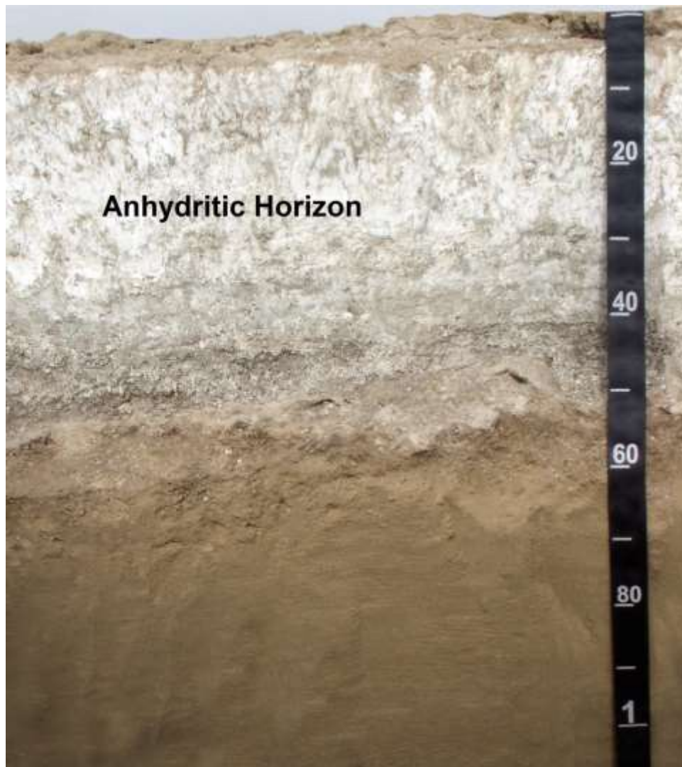
Profile of a soil in the United Arab Emirates that has an anhydritic horizon (white layer at a depth of 0 to about 60 cm). Depth is in cm. (Photo courtesy of Dr. Shabbir A. Shahid)
