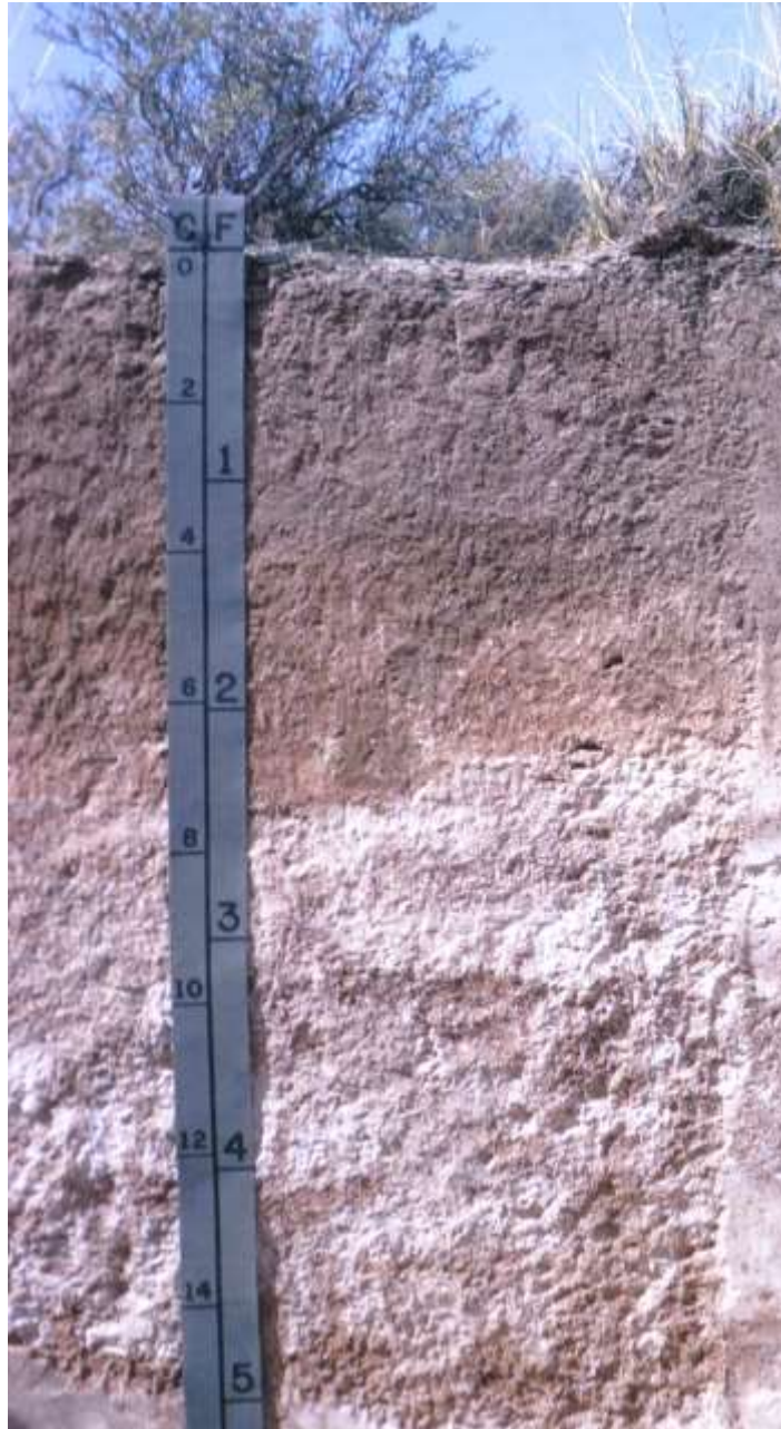
Profile of a soil in New Mexico. A calcic horizon is below a depth of about 75 cm. The white color is due to calcium carbonate concentrations. Scale is in decimeters (left) and feet (right).
